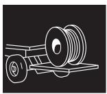
Lower reels from truck using hydraulic gate, hoist or fork lift.
