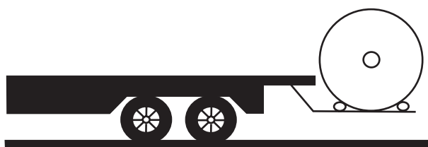
Reels should be lowered using hydraulic gate, hoise or forklift. LOWER CAREFULLY.
